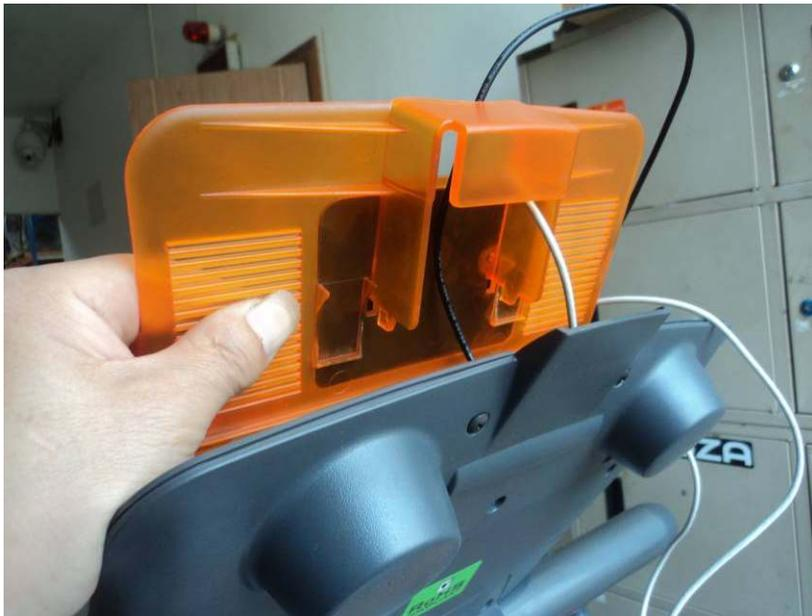
Audio input connection cable and USB connection cable need to pull out form mediaport housing
