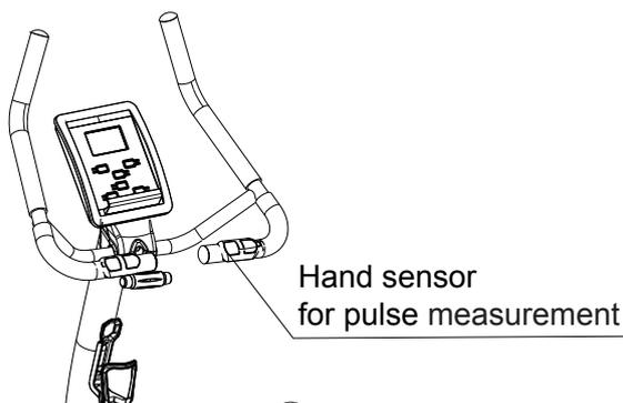
You can measure your pulse with the two hand sensor on the handle.
