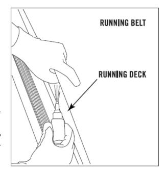
running deck. Tighten both rear roller bolts (matching up the marks for proper position) to original position. After you have applied lubricant, plug in the power cord, insert the safety key, start the treadmill and walk on the belt for two minutes to spread the lubricant.
